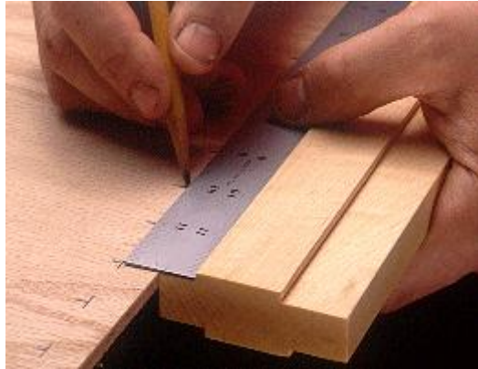
A layout tool helps when marking many screw holes all inset the same distance. It can be used to mark four different-size insets.
